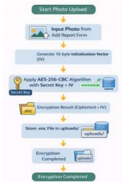
Figure 3. AES 256 Encryption Process Diagram
