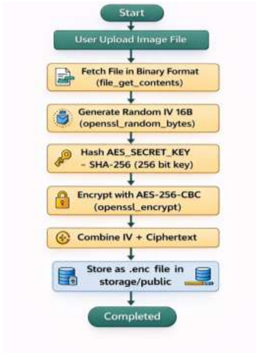
Figure 7. AES-256-CBC encryption process flow on the system
