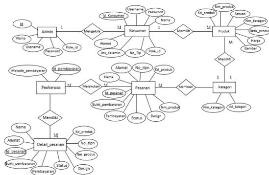
Gambar 5. Entity Relationship Diagram (ERD) Sistem Usulan
