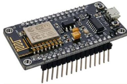
Sumber: (NodeMCU ESP8266 Pinout, Specifications, Features & Datasheet, n.d.)
